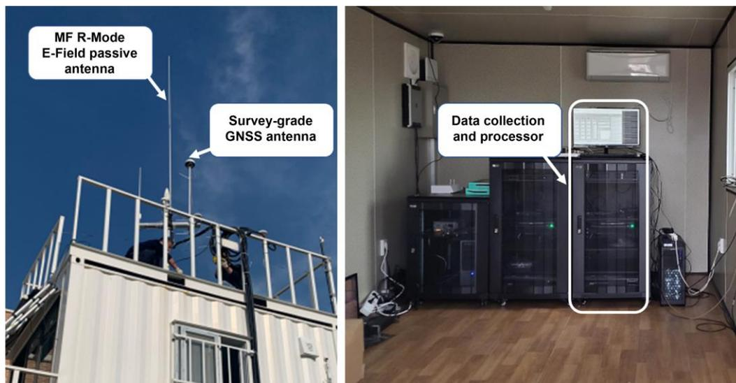
**Figure 2.** Installation of equipment at CORS to collect and monitor MF R-Mode signals. MF R-Mode E-field passive antenna and survey-grade GNSS antenna on the rooftop (left), Serco's MF R-Mode receiver (MFR-1a), and display devices in the shelter (right).
