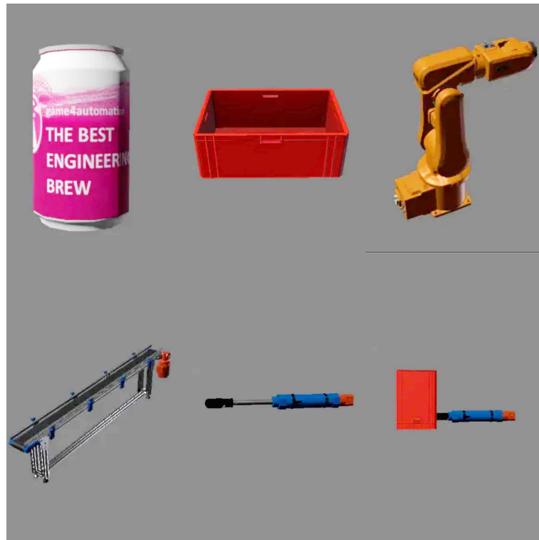
Figure 17. From the upper left corner are the can, box, robot, conveyor belt, piston, and slider.
