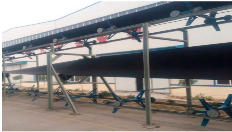
Figure 5. Conveying section of prototype rail conveyor.
