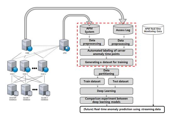
**Figure 1.** Process of constructing a deep learning dataset for anomaly detection in actual information systems.
