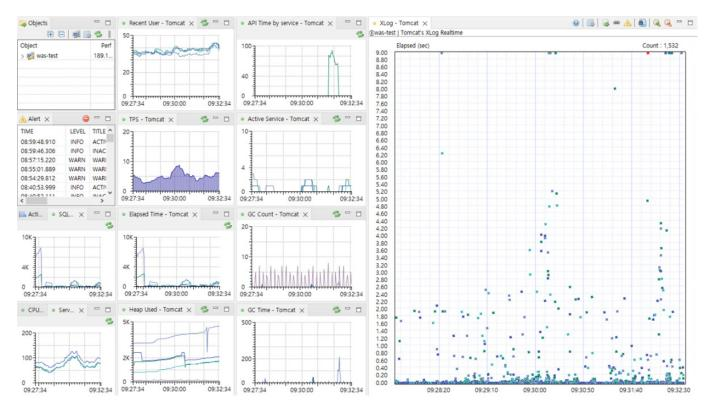
**Figure 2.** Monitoring dashboard of ScouterAPM, an open-source performance monitoring software. Ten types of performance monitoring data (lines) and response time based on user requests (dots).
