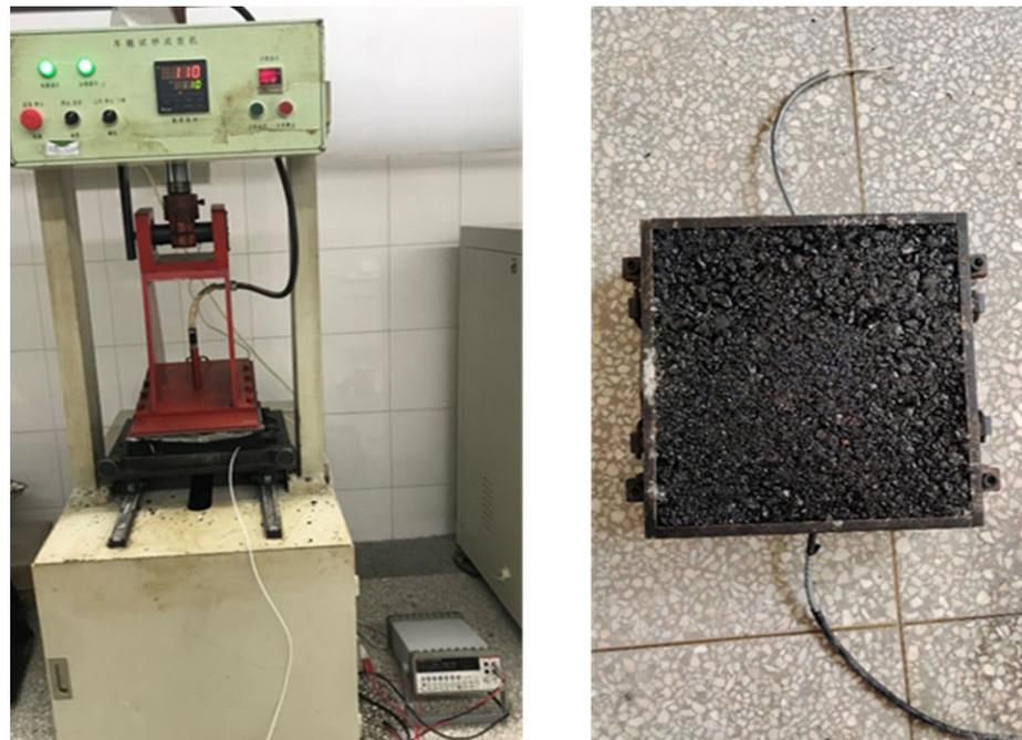
**Figure 6.** The embedment of piezoresistive sensors and formation of rutting slab.
