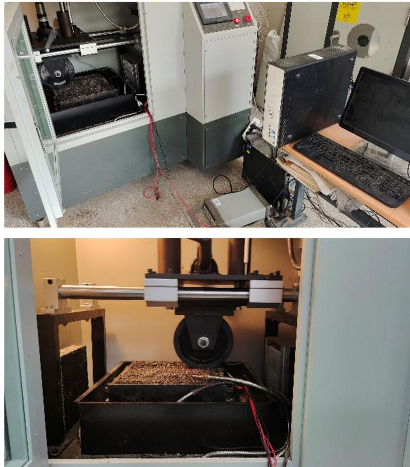
**Figure 8.** Rutting experiment for axle load sensor.
