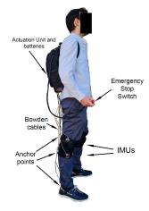
Figure 1. Prototype exosuit based on synergies.
