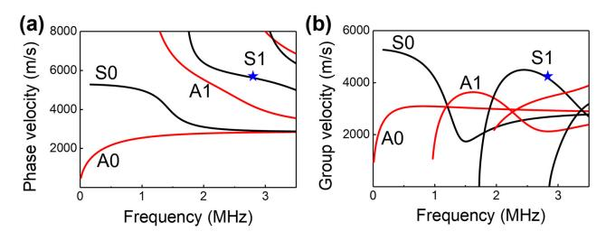
**Figure 1.** Dispersion curves of an aluminum alloy plate with a thickness of 1.6 mm, phase velocity (**a**) and group velocity (**b**) versus frequency.
