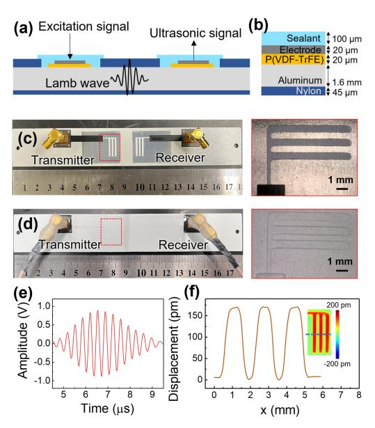
**Figure 2.** Schematic showing (**a**) coupon structure and (**b**) thickness of the layers, (**c**) photo of the coupon after coating P(VDF-TrFE) and electrodes, and (**d**) photo after coating a protective layer, (**e**) received ultrasonic signal measured via the pitch-catch mode, and (**f**) displacement versus location measured at 20 Vpp, 100 kHz; inset: effective d<sub>33</sub> mapping, measured with LSV.
