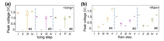
**Figure 7.** Boxplot graphs showing the mean, maximum, minimum, 25, and 75% values of the peak voltage of the ultrasonic signals at each stage of (**a**) icing (*i*: initial stage, *ii*: during icing, *iii*: melted ice, and *iv*: dried) and (**b**) rain test (*i*: initial stage, *ii*: during raining, *iii*: stop raining, *iv*: remove water, and *v*: dried), for test coupons #4, #5, and #6.
