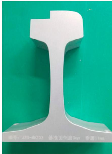
**Figure 14.** Standard worn rail with a vertical wear of 11.00 mm. (NO. JZG-MHZ02, horizontal wear 0 mm, vertical wear 11 mm).
