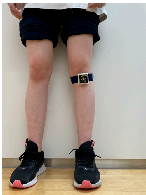
Figure 1. Photograph of the inertial measurement unit attached to the tibia.
