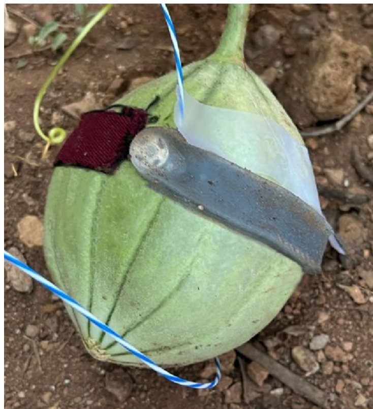
Figure 4. Graphical representation of the sensor positioning on the tested melon in the open field.
