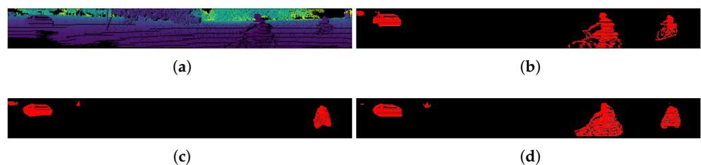
**Figure 5.** Qualitative results of different post-processing methods for MOS on the validation set, where red pixels correspond to moving objects (range view images). (a) Range Image; (b) Ground Truth Labels; (c) CRF; (d) KNN.
