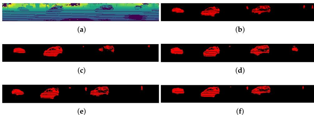
**Figure 3.** Qualitative results of different methods on the SemanticKITTI test set, where red pixels correspond to moving objects (range view images). (a) Range Image; (b) Ground Truth Labels; (c) BiSeNet (retrained); (d) SalsaNext (retrained); (e) LMNet; (f) ours.
