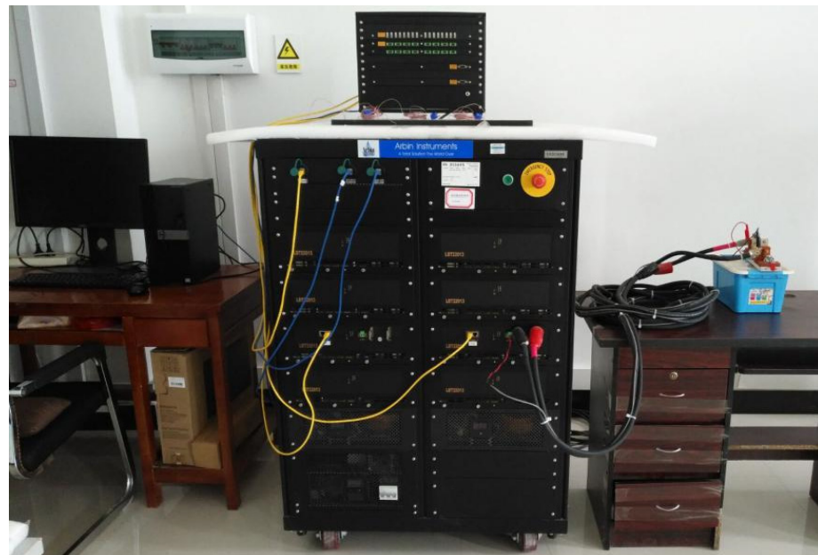
Figure 2. Arbin test rig and NCM532 lithium-ion batteries.
