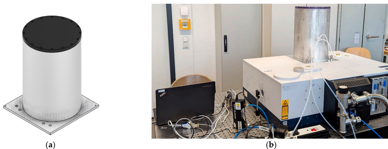
Figure 2. (a) CAD model of the designed lid. An aluminum cylinder (250 mm \times 15 mm \times 360 mm) with a polycarbonate plate (250 mm \times 15 mm) was fixed with screws to a rectangular aluminum plate (282 mm \times 293 mm \times 10 mm). (b) Measurement setup with the lid fixed to the FTIR spectrometer with the long-path gas cell inside. The gas inlet was connected to one of the bulkhead fittings on the outside of the lid, and a second bulkhead fitting was connected to the gas exhaust. The inlet and the outlet of the long-path gas cell were connected to the respective bulkhead fittings on the inside of the lid.
