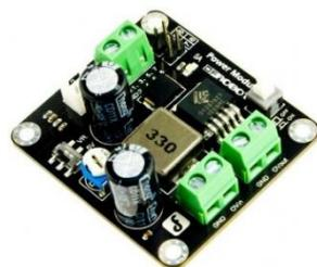
**Figure 6.** DFRobot 5-A Power Module DFR0205.
