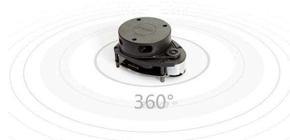
**Figure 3.** RPLIDAR A1M8 (2D rotating laser scanner).
