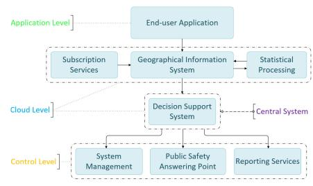
**Figure 2.** Description of the structure of the proposed system. It consists of three functioning levels: the application, the cloud, and the control level, with subsystems operating at their corresponding level.
