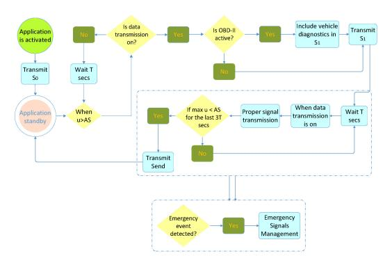
Figure 3. Description of how the mobile app operates in the application level.
