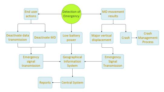
**Figure 4.** Description of what happens when the system detects an emergency (emergency signals management introduced in Figure 3).
