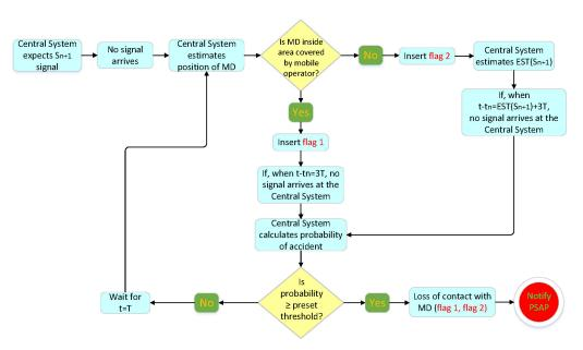
Figure 9. Description of what happens when the system loses contact with MD.
