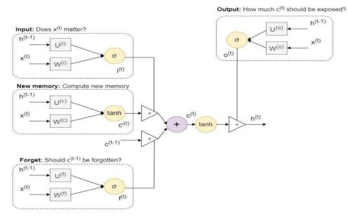
Figure 7. The structure of the LSTM technique.
