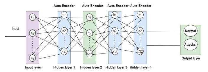
Figure 9. The structure of the auto-encoder (AE) model.
