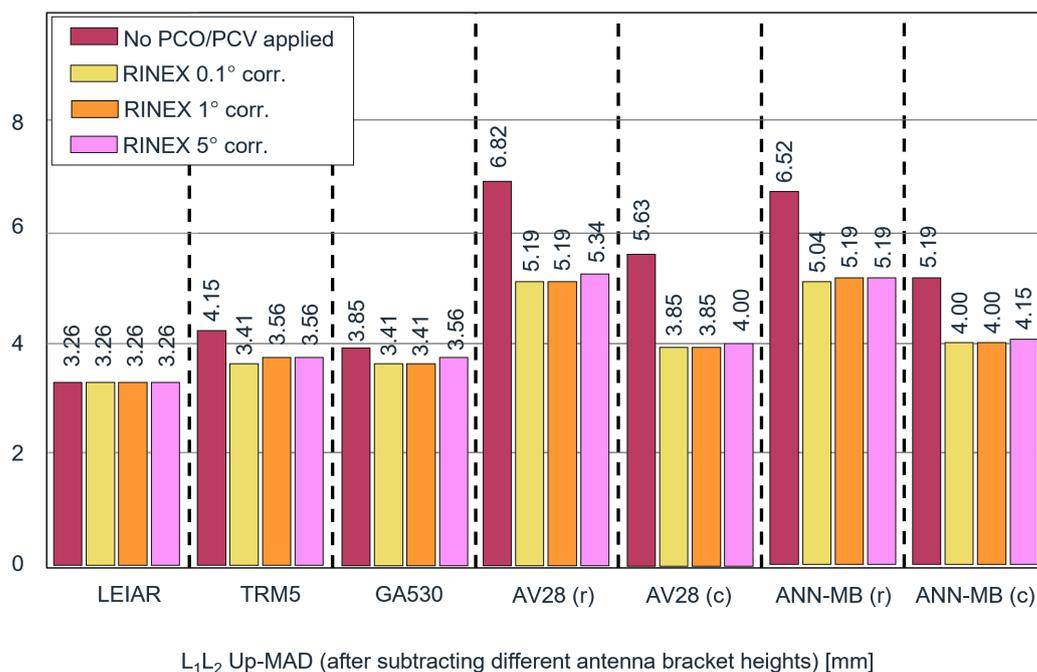
**Figure 6.** RTKLIB PPK MADs of the Up component of the kinematic positions before and after input data correction. The abbreviations (c) and (r) in the antenna names correspond to the utilized mounting brackets (circular plane and rectangular bracket).
