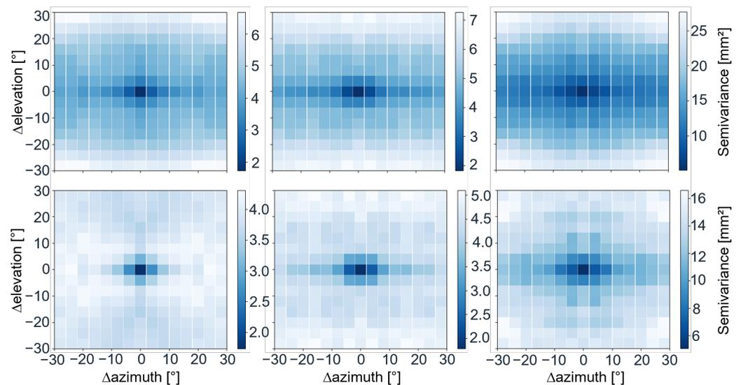
**Figure 3.** The 2D variogram maps of the residuals for the antennas TRM5 (left), AV 28 circular ground plane (middle), and AV28 rectangular adaptor (right), before (top) and after (bottom) removing the elevation pattern.
