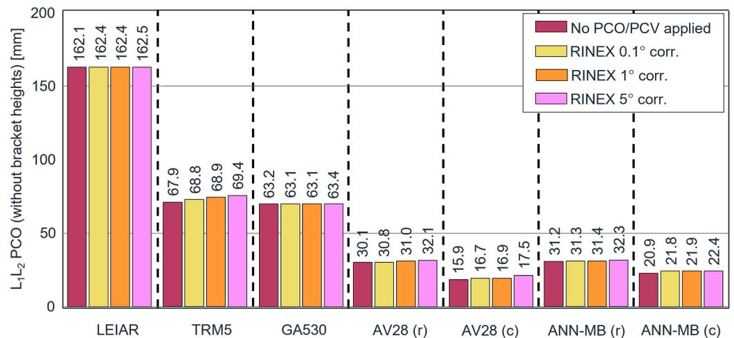
**Figure A3.** PPK estimated  $L_1 + L_2$  Up-component offsets. The abbreviations (c) and (r) in the antenna names correspond to the utilized mounting brackets (circular plane and rectangular bracket).
