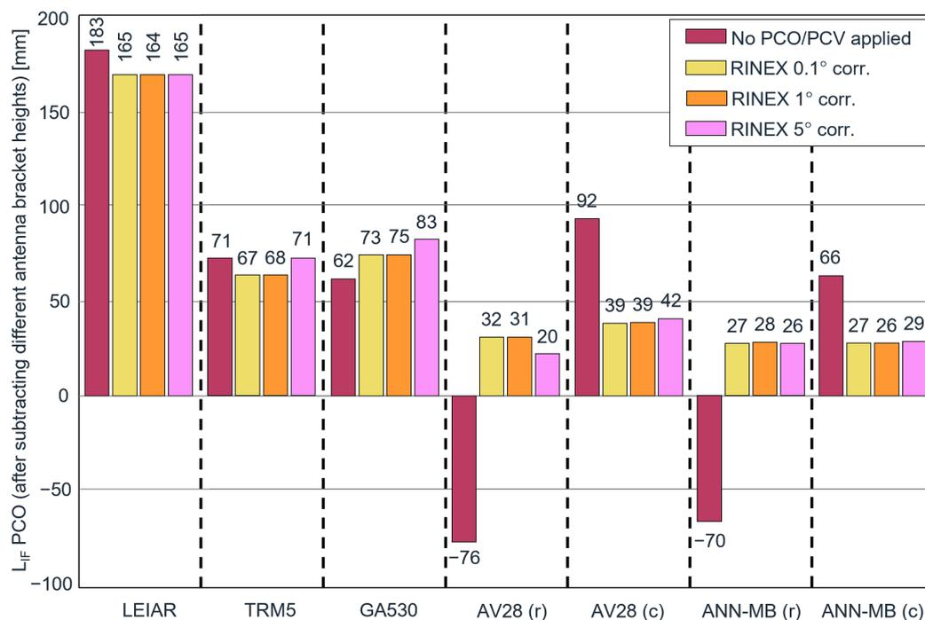
**Figure 5.** PPP height differences regarding the reference height before and after applying the PCV corrections. The abbreviations (c) and (r) in the antenna names correspond to the utilized mounting brackets (circular plane and rectangular bracket).
