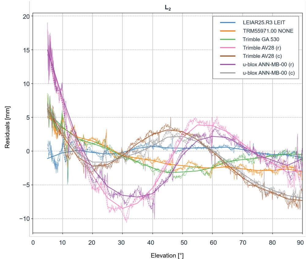
**Figure A2.** Elevation-dependent residuals on  $L_1$  (top) and  $L_2$  (bottom). The thin lines show the residuals obtained with a  $0.1^\circ$  averaging bin size, the thin dashed lines with  $1^\circ$  averaging bin size, and the thick lines the  $5^\circ$  averages. The terms (r) and (c) correspond to the utilized mounting brackets (circular plane and rectangular bracket).
