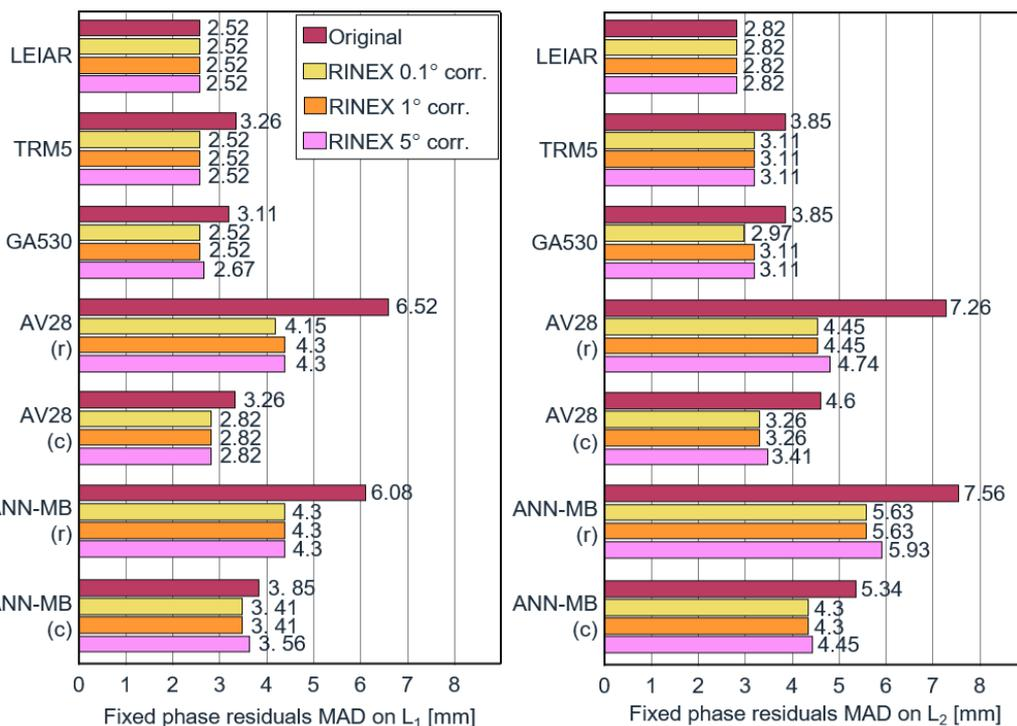
**Figure 2.** Ambiguity-fixed phase residuals on  $L_1$  (left) and  $L_2$  (right) before and after the calibration using 0.1°, 1°, and 5° binning widths. The abbreviations (c) and (r) in the antenna names correspond to the utilized mounting brackets (circular plane and rectangular bracket).
