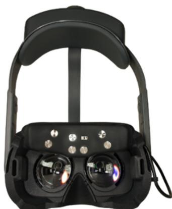
**Figure 3.** The emteqPRO Mask installed into the Pico Neo 2 Eye Virtual Reality (VR) headset.
