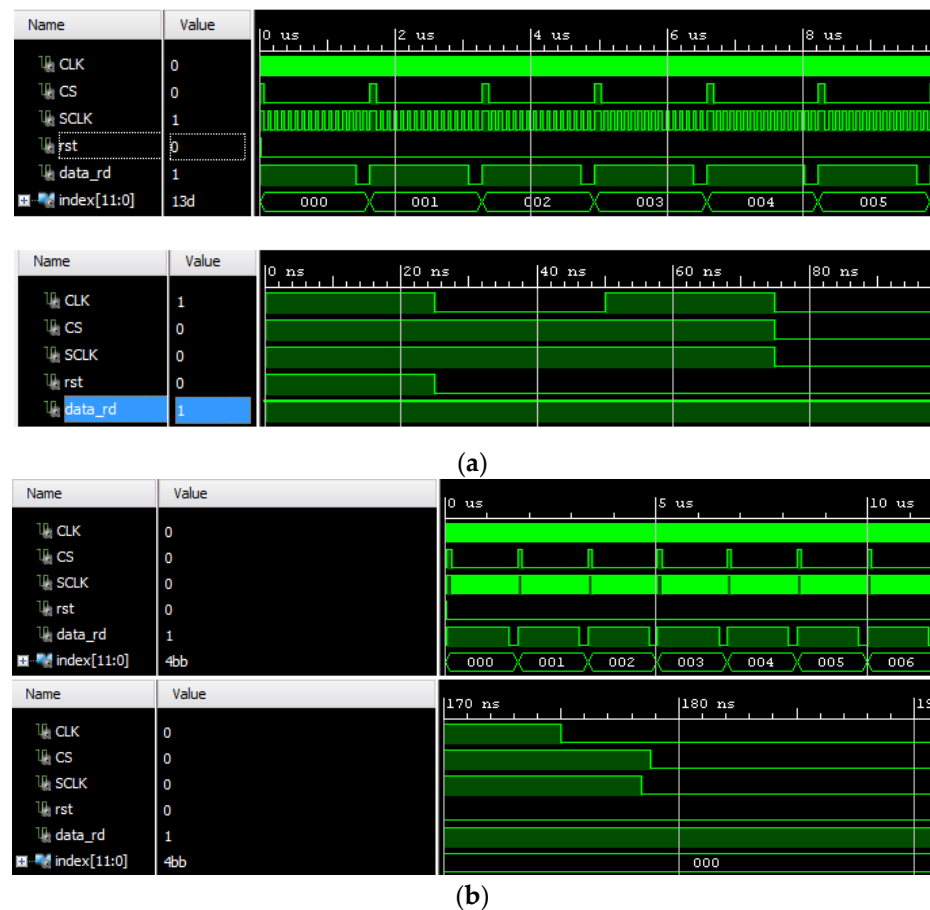
Figure 17. Simulation of VHDL code. (a) Prior synthesis process; (b) After synthesis process.
