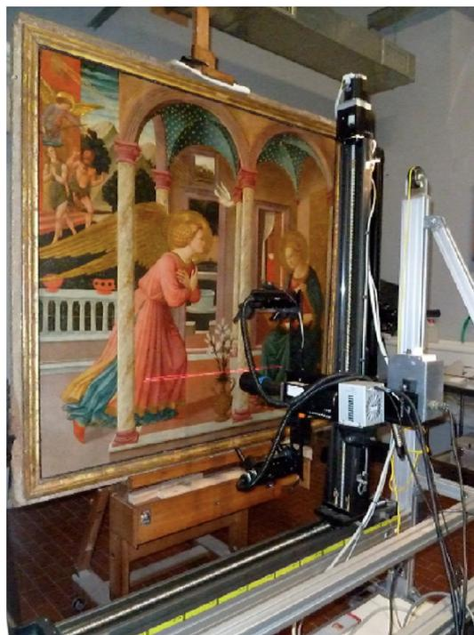
**Figure 1.** L'Istituto di Fisica Applicata “Nello Carrara” (IFAC-CNR), Florence, Italy, reflectance hyperspectral imaging system (400 to 1700 nm). Reprinted (adapted) with permission from [27]. Copyright 2016 American Chemical Society.
