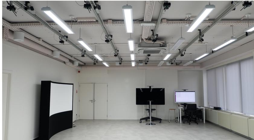
**Figure 1.** The proposed distributed VSN system, with 16 raspberry-pi cameras on the ceiling and a central service on the computer.
