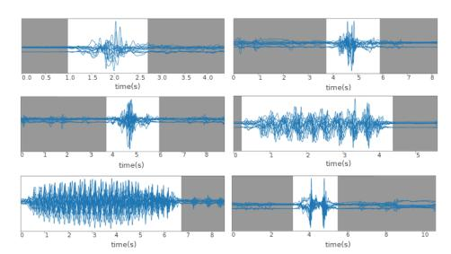
**Figure 3.** Examples of periods of high activity (white background) obtained after applying Algorithm 1. The examples show accelerometer data related to a shot, pass, pass, jog, sprint, and jump.
