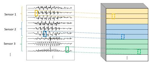
Figure 7. 1DCNN per sensor convolution logic.
