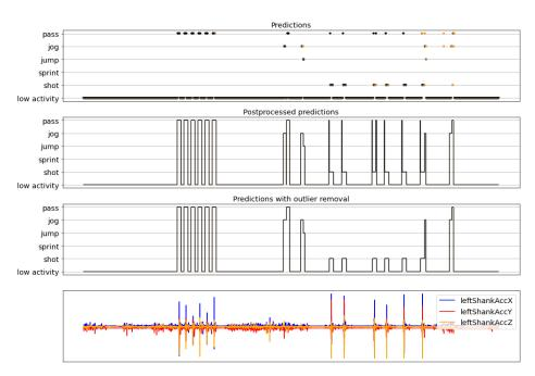
**Figure 21.** Example 3 of final results. True labels: 6 jumps-passes followed by 6 shots. Fast, unplanned movements are identified before and after the shots.
