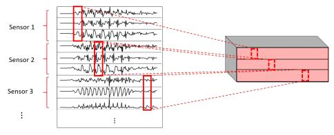
Figure 9. 2DCNN weight sharing logic.
