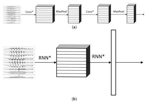
**Figure 5.** General CNN and RNN sub-networks for the models that combine CNNs and RNNs. The asterisks on the Conv layers mean the usage of different variations of CNNs. The asterisks on the RNN layers represent either LSTMs or bidirectional LSTMs. (FC = Fully Connected Feed Forward Neural Network.) (a) General CNN sub-network for the models that combine CNNs and RNNs. (b) general RNN sub-network for the models that combine CNNs and RNNs.
