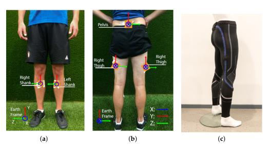
**Figure 1.** (a,b): Location of IMUs in experiments. Taken from [28]. (c): New sensor tights prototype with fully embedded sensors. Taken from [29].
