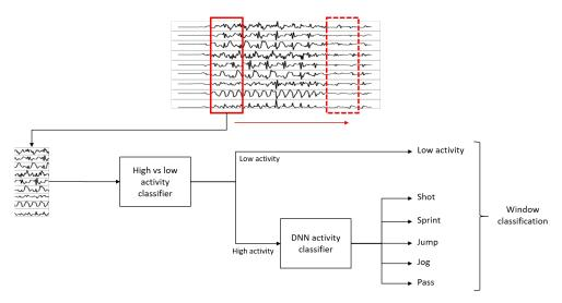
Figure 13. Sliding window evaluation diagram.
