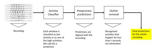
Figure 17. Complete sliding-window evaluation procedure.
