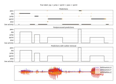
**Figure 19.** Example 1 of final results. True labels (in order): jog, jump, sprint, pass, and sprint with low activity periods in between each one of them. For the activity prediction plot, the orange-black color code of the dots and lines in the predictions represents the confidence of the predictions, where orange means low confidence and black high.
