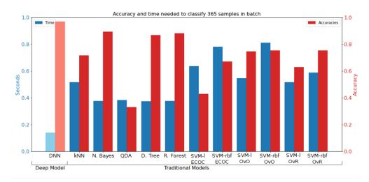
**Figure 18.** Prediction accuracy and evaluation time for traditional models in comparison to a deep learning-based model (DNN). The blue bars (left vertical axis) represent evaluation time and the red bars (right vertical axis) the prediction accuracy. The names of the models can be found in the main text.
