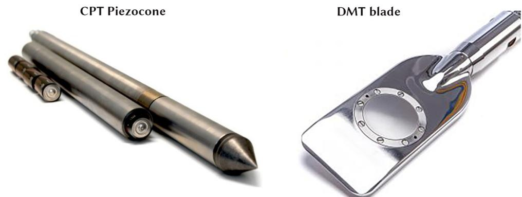
**Figure 3.** CPT piezocone cone and flat dilatometer DMT blade.
