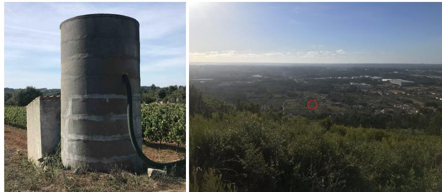
**Figure 11.** Structure used as target (left) and one of the photos used in the georeferencing procedure, with the target marked with a red circle (right).
