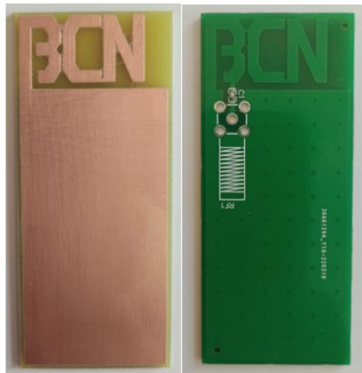
**Figure 9.** Fabricated PIFA antenna used in laboratory experiments (left) and prepared for the prototype testing (right).
