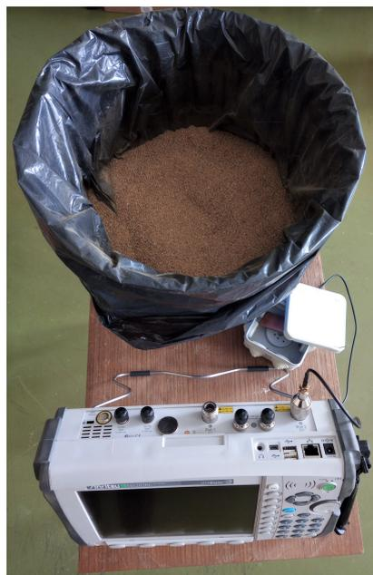
**Figure 10.** Setup for reflection measurements of antenna characteristics buried in sand.
