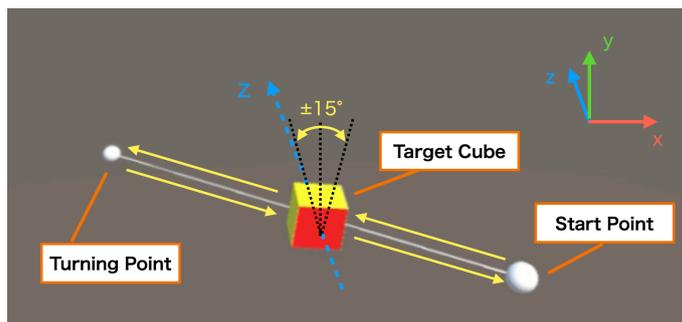
**Figure 4.** Movement of the target cube: The target cube makes one round trip on a line segment connecting two different points (start point and turning point) in virtual space, taking approximately 15 s. At the same time, the cube repeatedly rotates  $\pm 15^\circ$  around the z-axis in 2 s per round trip.
