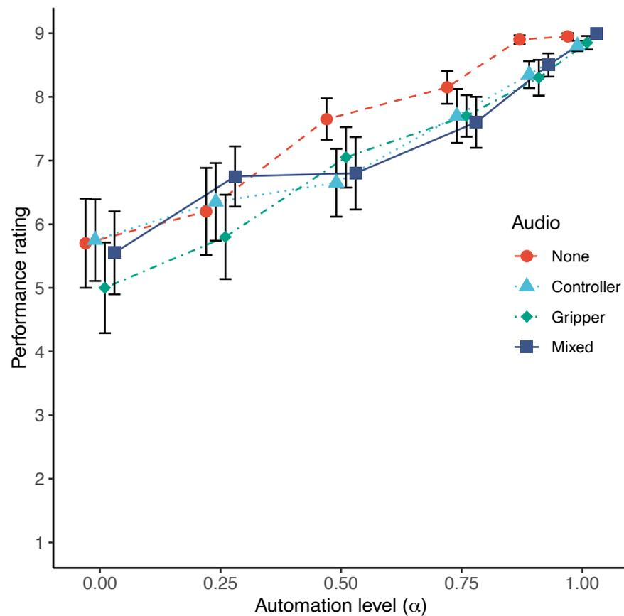
**Figure 7.** Mean performance ratings at each level of automation under four different auditory feedback conditions. Error bars represent standard errors. Performance rating increases with increasing level of automation.
