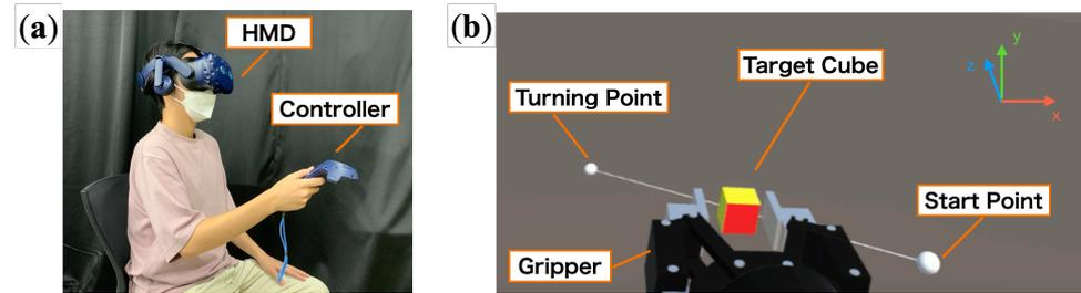
**Figure 2.** Experimental setup: (a) The operator wears the HMD while sitting on a chair and holds the controller in his right hand. (b) An image of the operator's viewpoint displayed on the HMD.
