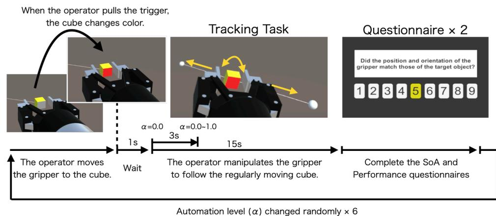
**Figure 5.** Procedure for one set of the tracking task.
