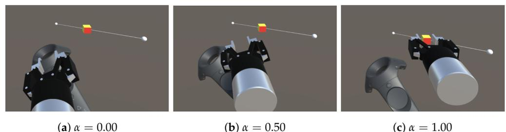
**Figure 3.** Position and orientation relationships between controller, virtual gripper, and target cube: (a) The gripper synchronizes with the controller. (b) The position and orientation of the gripper are between the controller and the target cube. (c) The gripper synchronizes with the target cube. In these figures, the controller model is shown for comparison but was not used during the experiment.
