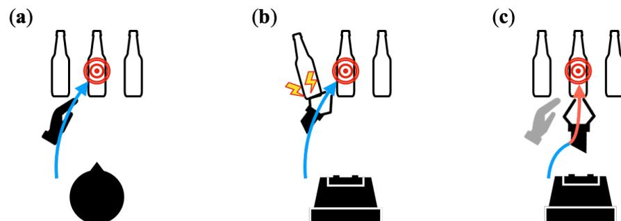
**Figure 1.** Shared control of grasping assistance to resolve differences in human and robot physical structures: (a) Humans plan movements based on information about their own physical structure. (b) When robots are manually and remotely operated by humans, differences in the physical structures of humans and robots reduce operability. (c) Shared control, which fuses control commands from humans and robots, supports task execution.
