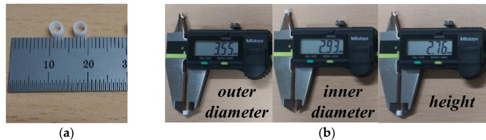
**Figure 11.** Fabricated liquid container: (a) photograph and (b) measured dimensions.
