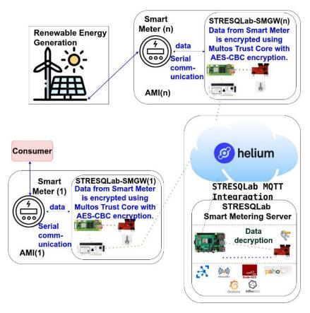
Figure 17. Block diagram of the IoT system.
