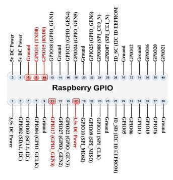
Figure 19. GPIO used by the module.
