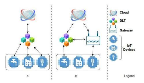
Figure 4. DLT and IoT Integration schemas (a) Without a Gateway Device, (b) With Gateway Device.
