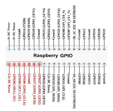
Figure 20. Multos Trust Core to pi GPIO.
