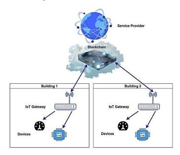
Figure 3. AMI-Blockchain Application Architecture.
