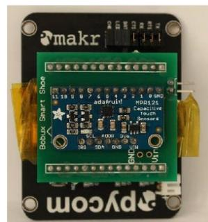
**Figure 15.** PCB shield assembled on top of the Pycom Expansion Board.
