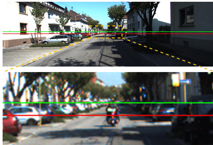
Figure 9. Visualization of vanishing lines. The red and green horizontal lines are vanishing lines converted from fixed and dynamic ground plane normals, respectively. The (bottom) image is a zoom-in image of orange rectangular areas from the (top) image. The green line is obviously a more accurate estimation of the vanishing line.
