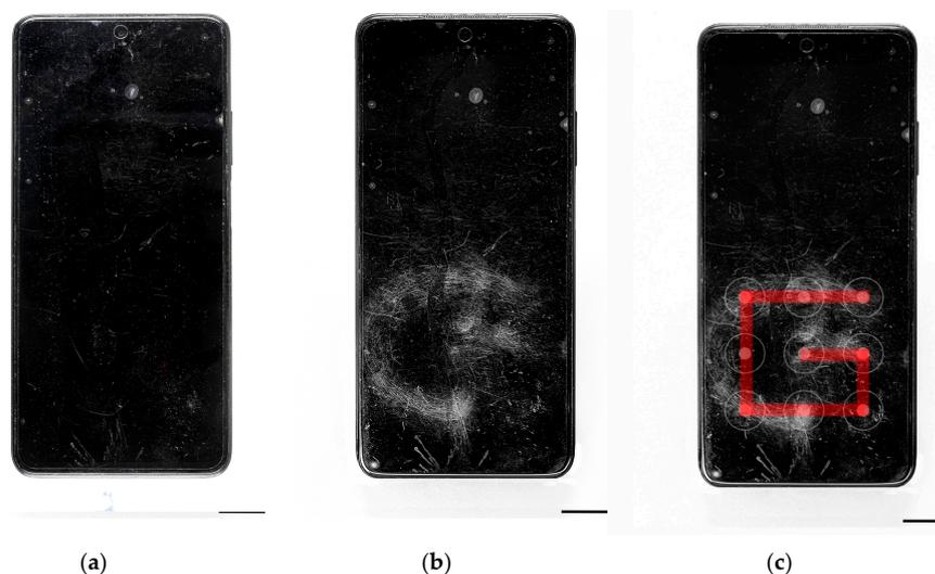
**Figure 8.** Images from a mobile phone photographed (a) with a conventional camera and illuminated with white visible light; (b) captured by Invespector camera and illuminated with IR radiation 950 nm; and (c) the pattern movement recovered to unlock the smartphone successfully.
