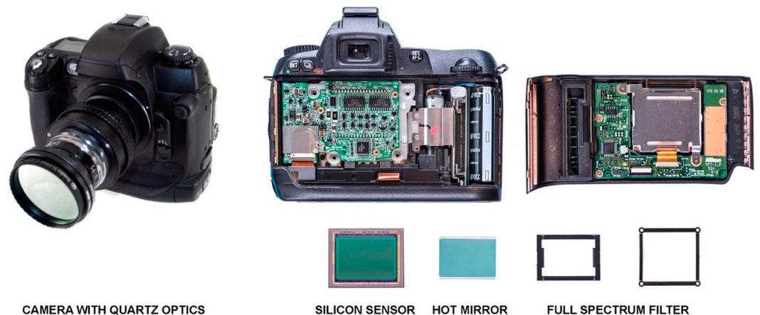
**Figure 2.** Multispectral capture device modified with quartz optics and Baader UV/IR-cut coupled.
