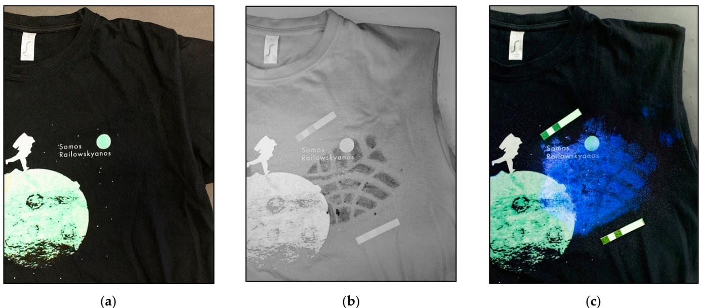
**Figure 4.** Images of black cotton shirt with traces of latent blood photographed (a) with conventional camera and illuminated with white visible light, (b) by Invespector illuminated with IR radiation 850 nm and (c) after applying a chemo locator, such as Bluestar.
