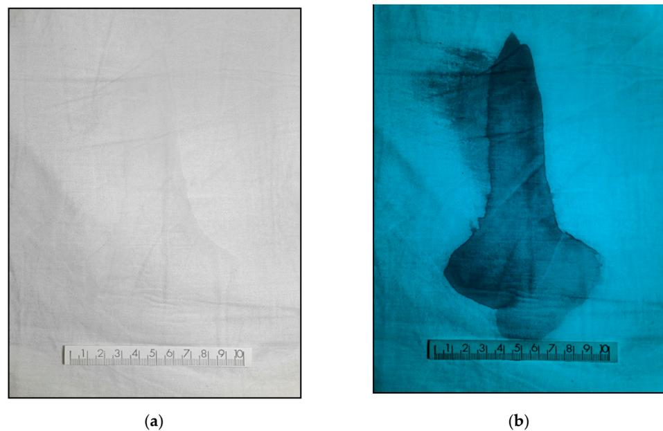
**Figure 7.** Images of a cotton sheet with traces of latent blood photographed: (a) with a conventional camera illuminated with white visible light and (b) Invespector system using UV illumination 365 nm.
