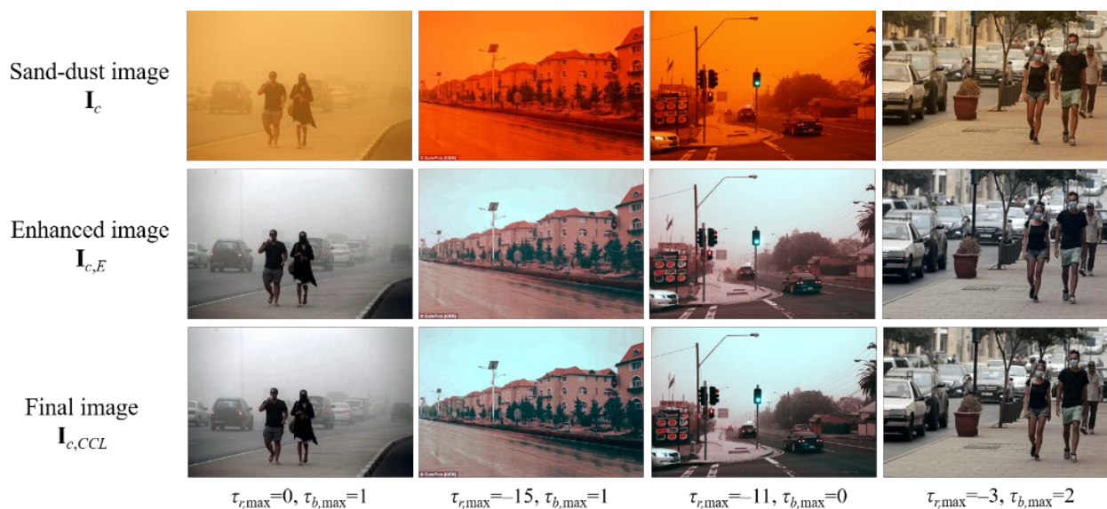
Figure 7. Fine-tuned images using a cross-correlation-based chromatic histogram shift.
