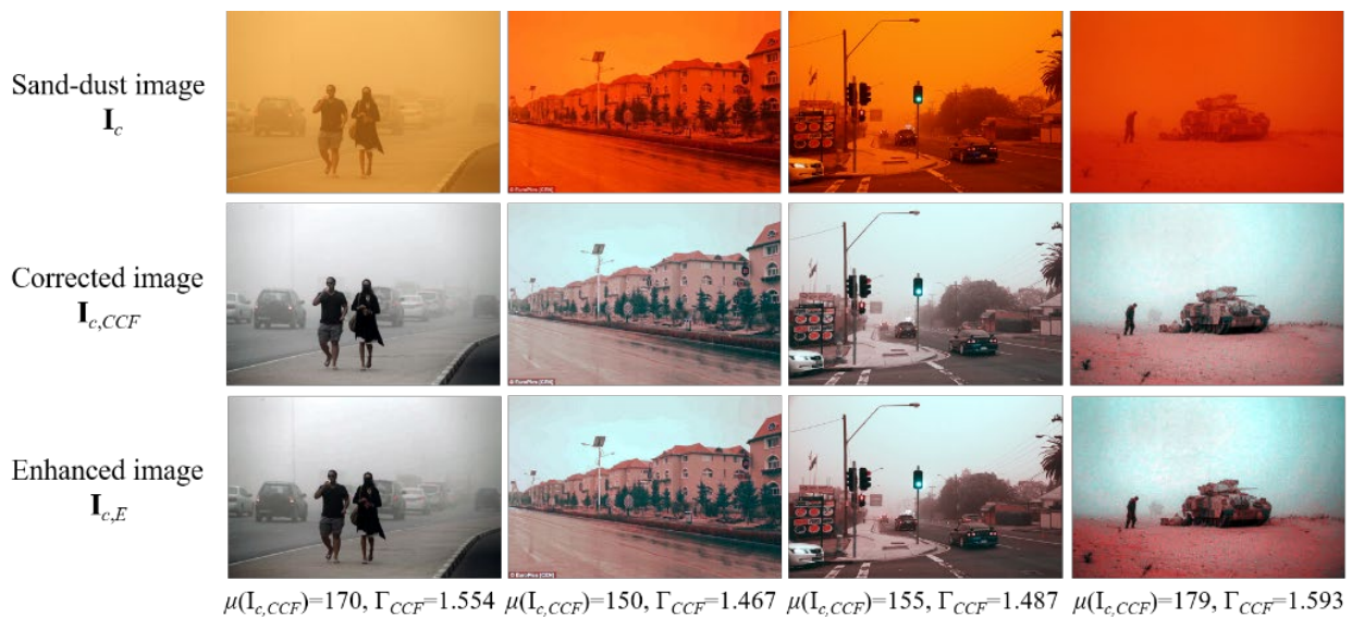
Figure 6. Enhanced images produced using the proposed dehazing method. Mean values of color-corrected images and corresponding gamma values are shown for \Gamma_{\max} = 2 .
