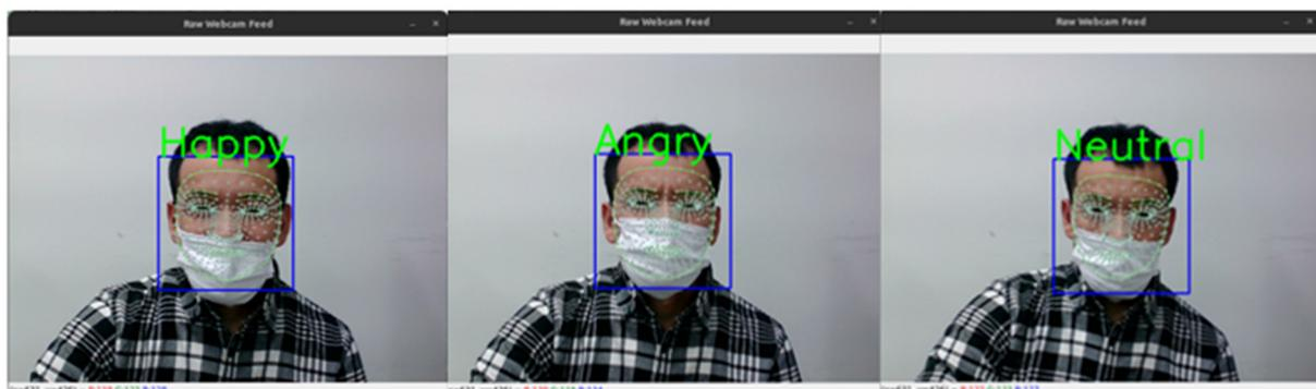
**Figure 11.** Haar-cascade face detection based real-time emotion recognition video capture.
