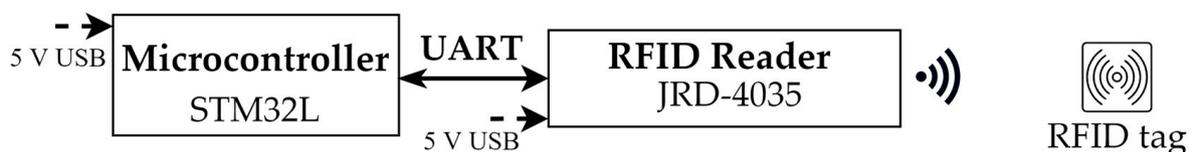
Figure 9. RFID gate access node block scheme.
