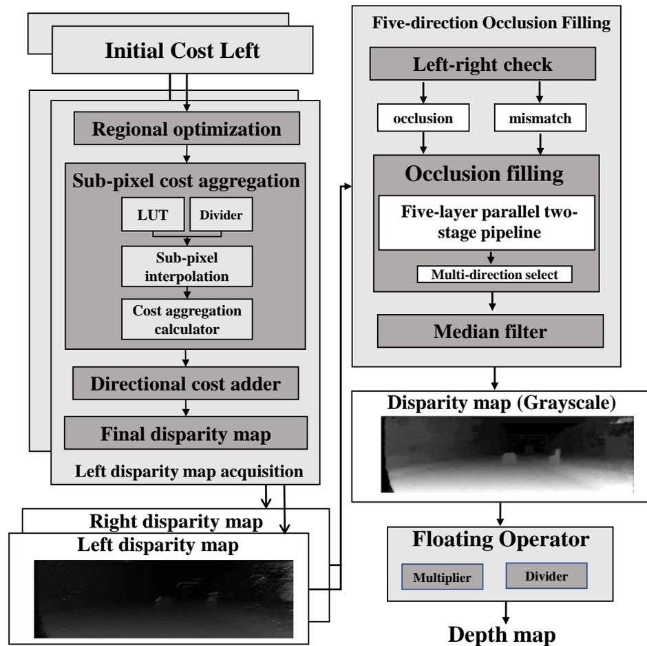
**Figure 7.** The hardware implementation for sub-pixel cost aggregation and five-direction occlusion filling.
