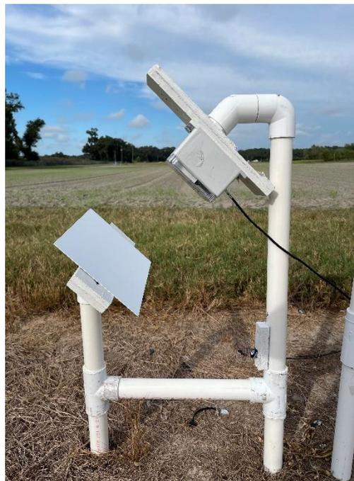
**Figure 4.** Reference surface and camera enclosure with the RGB camera at UF PSREU, Citra.
