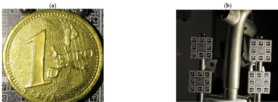
**Figure 1.** Examples of objects considered in this work and featuring non-collaborative surfaces (shiny, textureless). (a) a gold foiled surface shaped like a Euro coin featuring high reflective, very detailed structures [25]; (b) a metallic object with less reflectivity while featuring a geometrically complex shape [11].
