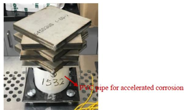
Figure 10. Experimental setup for combined loading–corrosion tests.
