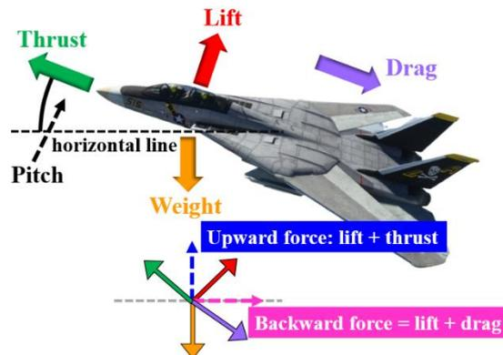
Figure 6. Four forces during takeoff.
