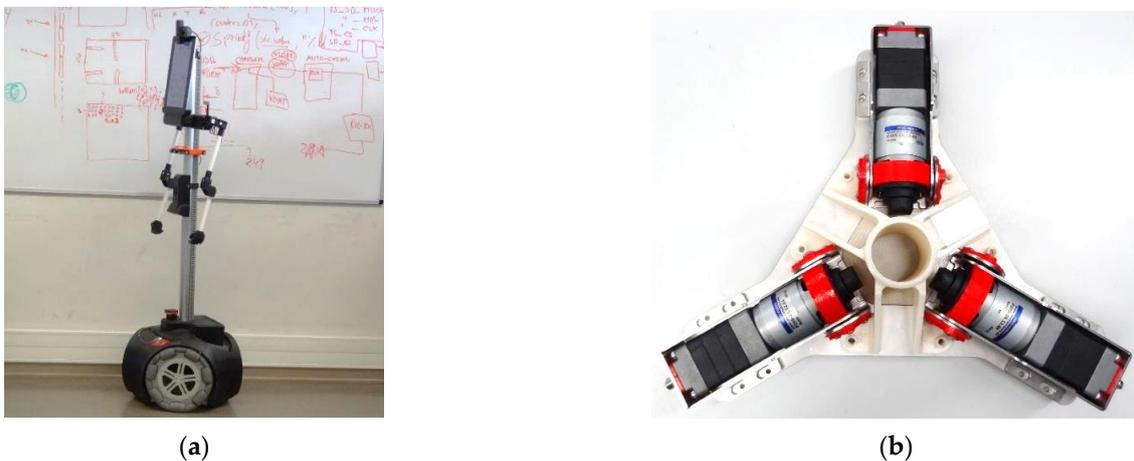
**Figure 1.** (a) Image of the APR-02 mobile robot. (b) Details of the internal structure supporting the three BDCMs that drive the three omnidirectional wheels of the mobile robot.
