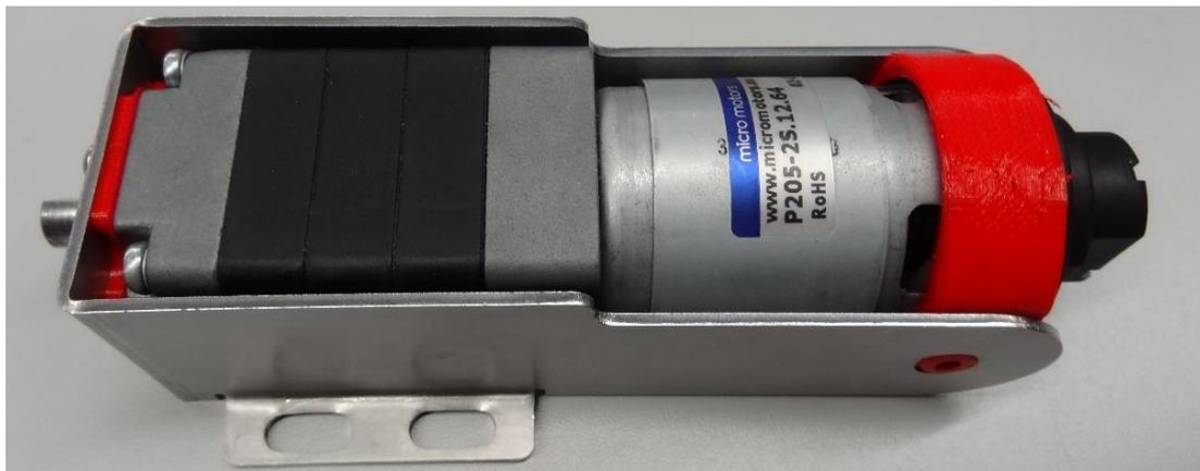
**Figure 2.** Image of the BDCM used in the APR-02 mobile robot, which includes a 64:1 planetary gearbox and a low-cost magnetic encoder attached to the motor shaft. The motor is supported by an aluminum support structure that has some (red) support elements made of flexible rubber in order to reduce the transmission of vibrations.
