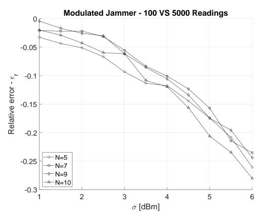
**Figure 7.** Comparison between 100 and 5000 readings of the jamming signal as a function of  $\sigma$  and the number of nodes.
