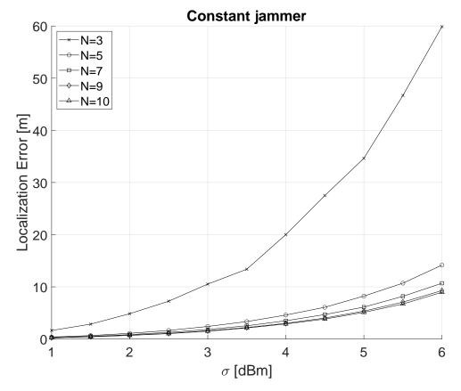
**Figure 4.** Localization of a constant jammer as a function of  $\sigma$  (1 dBm $\leq \sigma \leq$  6 dBm) and the number *N* of sensing nodes (3  $\leq N \leq$  10).
