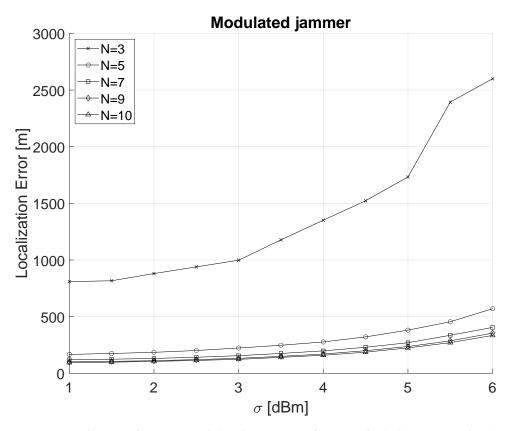
**Figure 5.** Localization of a power-modulated jammer as a function of  $\sigma$  (1 dBm $\leq \sigma \leq$  6 dBm) and the number *N* of sensing nodes (3  $\leq N \leq$  10).
