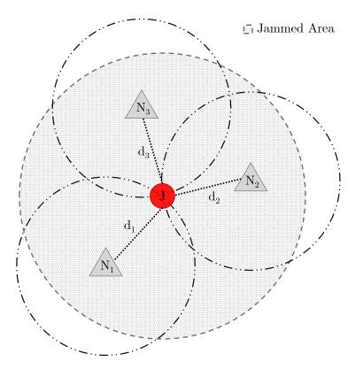
**Figure 2.** Jammer localization by three-lateration: 3 sensors collaborating to estimate the jammer position.
