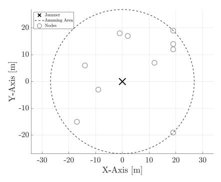
**Figure 1.** A typical random deployment: 10 nodes and the jammer (black cross) at the center of the scene. The black dashed circle represents the jamming area.
