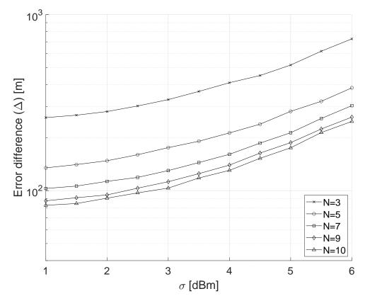
**Figure 6.** Comparison between the modulated-power and constant-power jammer: localization error as a function of  $\sigma$  while the number of nodes in the playground spans between N = 3 and N = 9.
