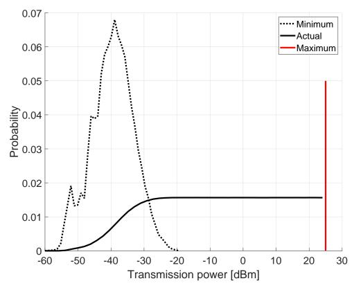
**Figure 3.** Power-modulated jammer: the minimum transmission power is opportunistically chosen in order cover the whole area.
