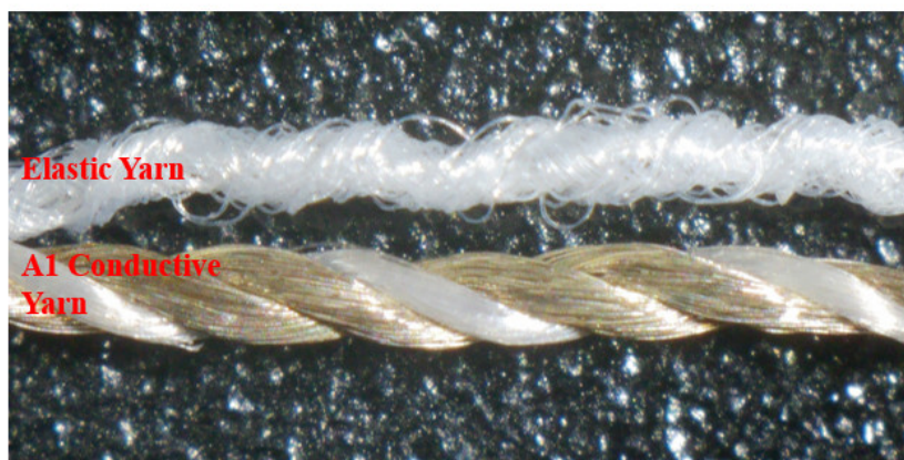
Figure S7. Optical image of plating elastic yarn (white) and A1 conductive yarn (white and silver).
