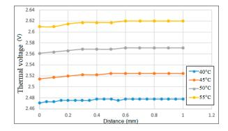
**Figure 11.** Correlation between thermal voltage and sensing distance for working temperatures in range of  $40 \sim 55$  °C.
