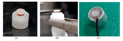
**Figure 7.** Photographs of the coil winding structure and the sensor assembly process: (**a**) coil winding, (**b**) wire connection, and (**c**) complete sensor assembly.
