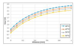
**Figure 10.** Correlation between output inductive voltage and sensing distance for working temperatures in the range of  $40 \sim 55$  °C.
