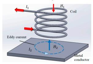
Figure 1. Schematic illustration of EC sensing principle.
