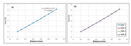
**Figure 9.** Correlation between output voltage and sensing distance over: (**a**) single test, and (**b**) four repeated tests.
