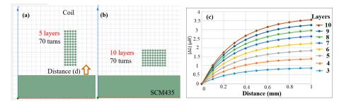
**Figure 4.** (**a**) Coil winding arrangement with 5 layers, (**b**) coil winding arrangement with 10 layers, and (**c**) effect of number of layers on inductance sensitivity.
