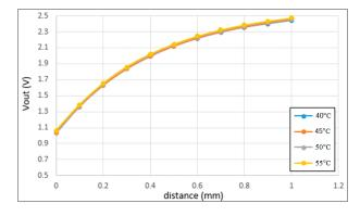
Figure 13. Correlation between output voltage and sensing distance following temperature compensation.
