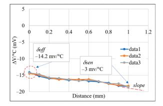
Figure 12. Correlation between temperature drift and sensing distance with no temperature compensation.
