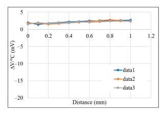
Figure 14. Correlation between temperature drift and sensing distance following temperature compensation.
