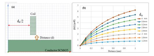
Figure 3. (a) Coil winding arrangement with 5 layers, and (b) effect of inner coil diameter on inductance.
