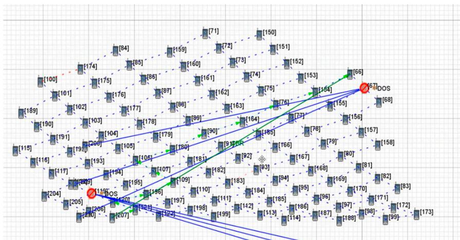
Figure 4. Two-satellite-key-node attack scenario under OSPFv2 protocol.
