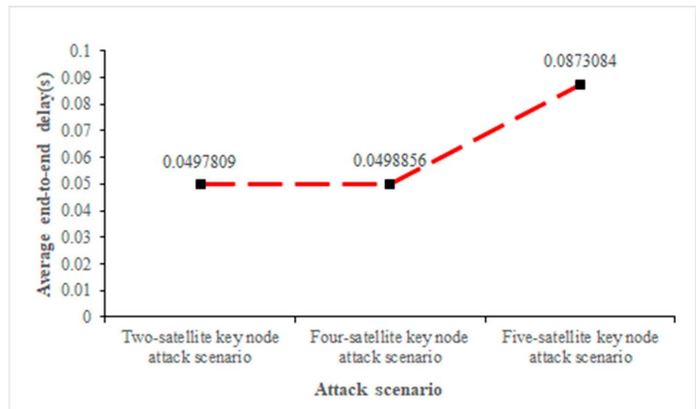
Figure 11. Average end-to-end delay under three attack scenarios.
