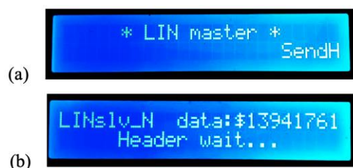
Figure 13. Initial states displayed after reset or power-on: (a) master node, (b) normal slave node.
