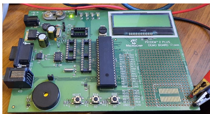
Figure 7. PICDEM development platform used for PIC18F performance testing.
