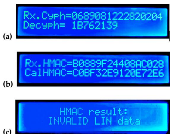
Figure 20. Master node's state after the attacked response; (a) decryption result; (b) HMAC result; (c) LIN data validity result.
