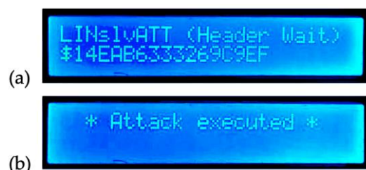
Figure 19. Attacking slave node's screen displays; (a) initial state, (b) result after response sent.
