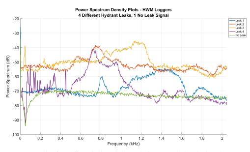
Figure 6. PSD plot: four different hydrant leak signals (loggers on leaking hydrants).
