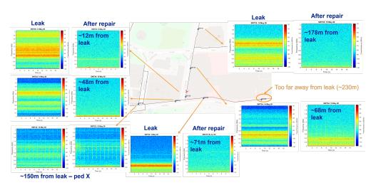
**Figure 5.** An illustration of a single leak source originating from a broken back pipe, and the noise spectrograms picked up by 6 HWM PermaNET+ loggers in the vicinity. The 7th sensor on the right is located too far away to pick it up.
