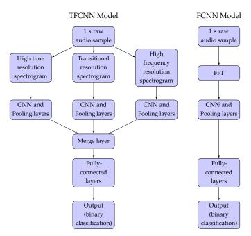
Figure 8. TFCNN and FCNN model structures.
