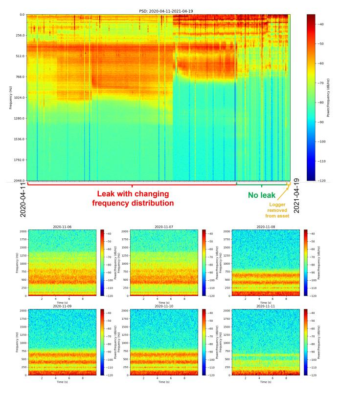
**Figure 7.** Leaking main tap-changing frequency distribution is visible in the PSD (**top**) and spectrograms (**bottom**) from consecutive days. The logger was situated approximately 59 m away from the leak location, with noise being propagated along a straight section of 150 mm diameter CICL pipe.
