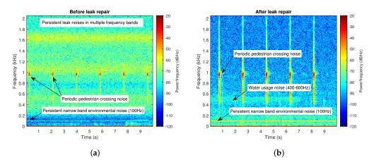
**Figure 4.** Spectrograms for a sensor detecting a variety of noises: (a) before and (b) after a leak was repaired  $\sim$ 21 m away from the sensor. The sensor was situated <1 m from a pedestrian crossing.
