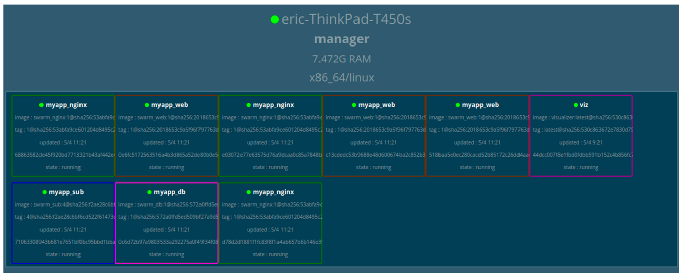
Figure 12. Docker Swarm with duplicated container services at the scale up purpose.
