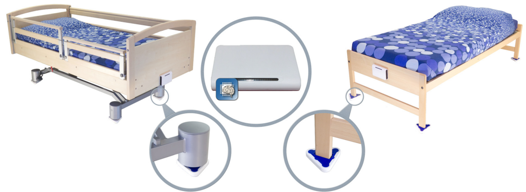
Figure 1. Human in bed monitoring through signals generated by sensors placed under the bed. Under each of the four bed legs, two sensors are placed: one weight sensor and one motion sensor. Thus, eight sensor measurement values are generated continuously over time for further processing by the anomaly detection intelligent system [25].
