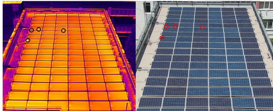
**Figure 8.** Thermal scanning using drone inspection displays the hot spot on the PV farm.
