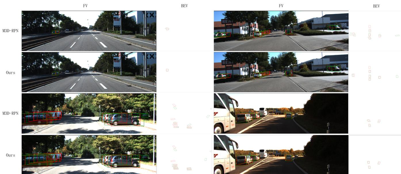
**Figure 12.** Qualitative results from our framework and MDSNet in the KITTI validation set. We use red box to denote the ground truth box and green box to denote the predicted box. It can be observed from the figure that our model has better accuracy for the prediction of depth and angle, and better performance for the detection of occluded objects.
